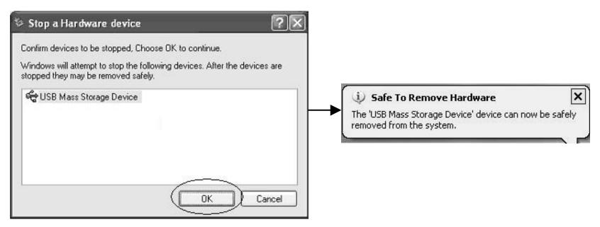
**Notice:** Never unplug the USB cable when transmitting data with PC to avoid damaging the Player; after data transmitting, please do not disconnect the player from PC until "Device now be safely removed" appears; while using USB function, all other buttons will be nonfunctional.
